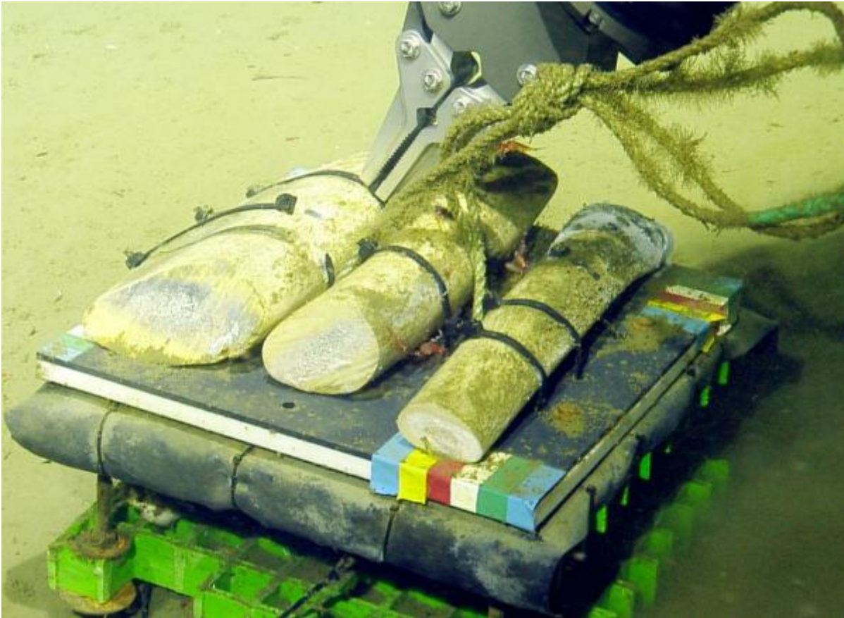
Hercules clipping the cable ties securing the whalebone to the experiment package.
