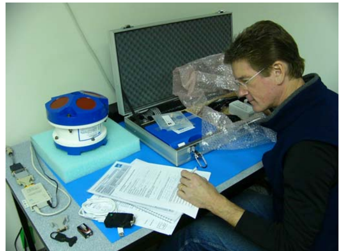
Kim Wallace of Highland Technologies reviewing testing protocols for a 1200kHz ADCP (Teledyne/RDI WorkHorse Monitor) to be deployed at Folger Passage.
