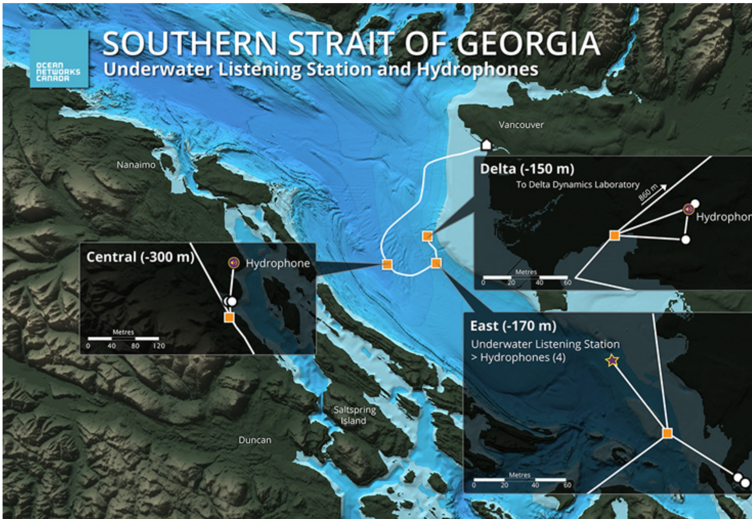
Figure 2. The underwater listening station and hydrophones in the southern Strait of Georgia deliver real-time acoustic measurements on marine mammal vocalizations and underwater vessel noise.
