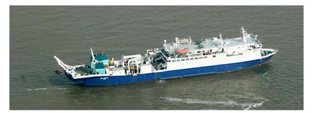
The Cable Ship (CS) Wave Venture, owned and operated by Global Marine Systems Ltd., deploys the eastern (shallow) Node base in the Strait of Georgia on May 5, 2007. The shallow (170m) Node represents the terminus of the 39 km of fibre optic cable laid in the Strait of Georgia, with a second (deep) Node to the west on the 300m isobath. The cable makes a shore landing at the south-east end of the lona Causeway. See inside for a complete story on the cable lay.
