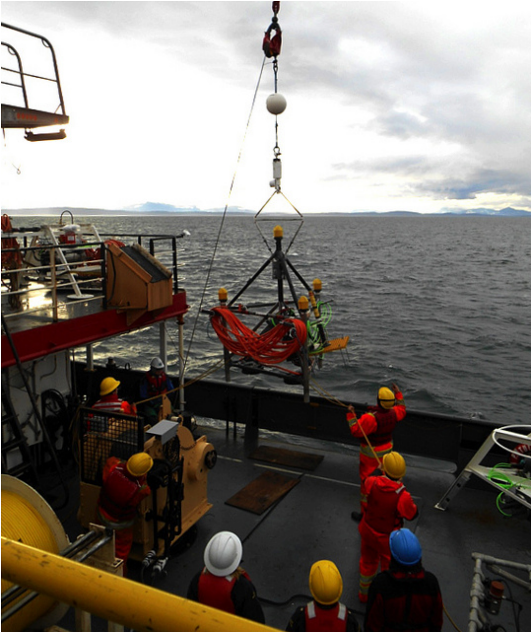
JASCO AMAR and hydrophone array being lowered to the seafloor at the VENUS observatory's Strait of Georgia East site (at 170 m depth).
