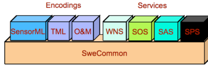
Fig. 1: Sensor Web Enablement family of protocols. This project proposes to implement the SOS data access services for a large subset of ONC Observatory's scalar sensors. Those sensors will be described using the SensorML markup language. Graphic courtesy of Simon Jirka, University of Münster.
