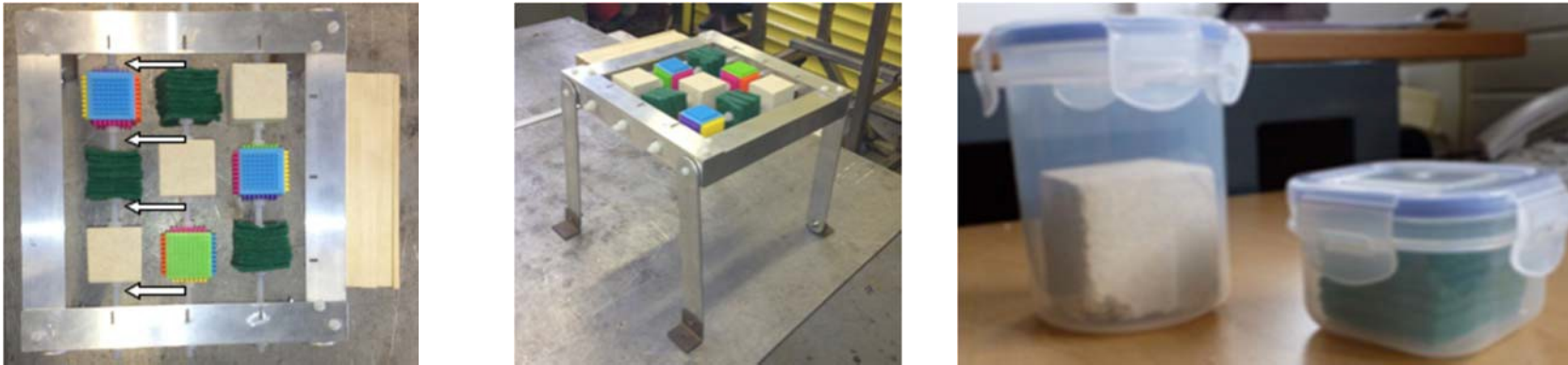
Figure 1. Cut between blocks with bolt cutters as indicated by the arrows (left). Image in the far right shows the tap-ware containers that will be provided, which will be pre-labelled (by substrate types and replicates) and pre-filled with Ethanol solution.
