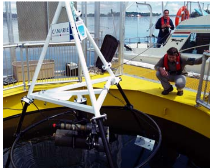
The HDTV Camera, part of the Oceans 2.0 project undergoes a test deployment in the Saanich Inlet, through UVic's Ocean Technology Test Bed ring buoy.
